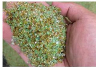
We installed Activated Filter Media composed of recycled green and amber glass in Balara Treatment Plant 2. This has resulted to less backwash water, efficient removal of iron and manganese that stains and restricts water flow and reduces water pressure, and reduced chlorine consumption.
